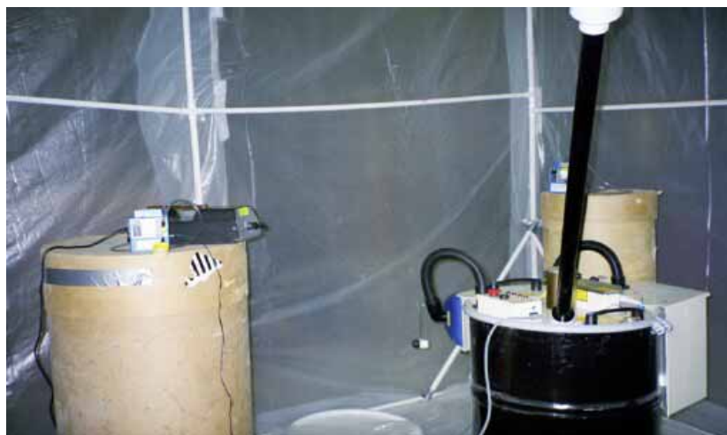
Photograph 3. 7: Placement of Air Sampling Pump & Jerome Analyzer in Relation to DTC Device
