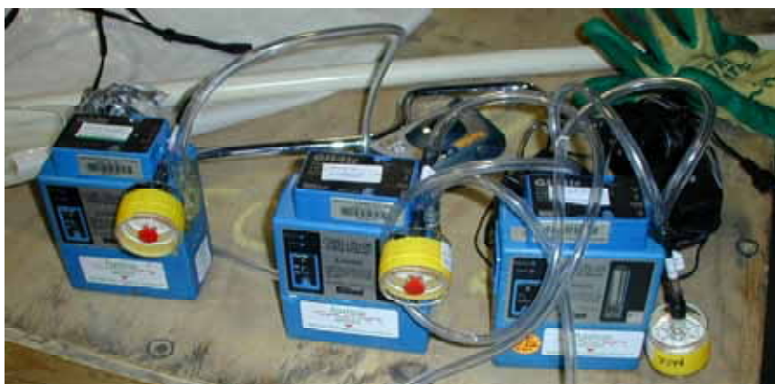
Photograph 3. 2: Sensidyne Air Sampling Pumps
